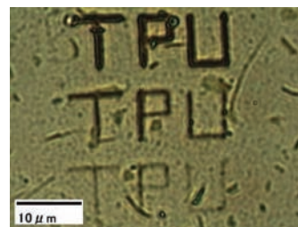
Figure 3. Micrograph of polypyrrole patterns on the glass substrate obtained by two-photon-sensitized polymerization with different driving rates of the laser focus (Top: 250 nm/s, Middle: 500 nm/s, Bottom: 1000 nm/s).
